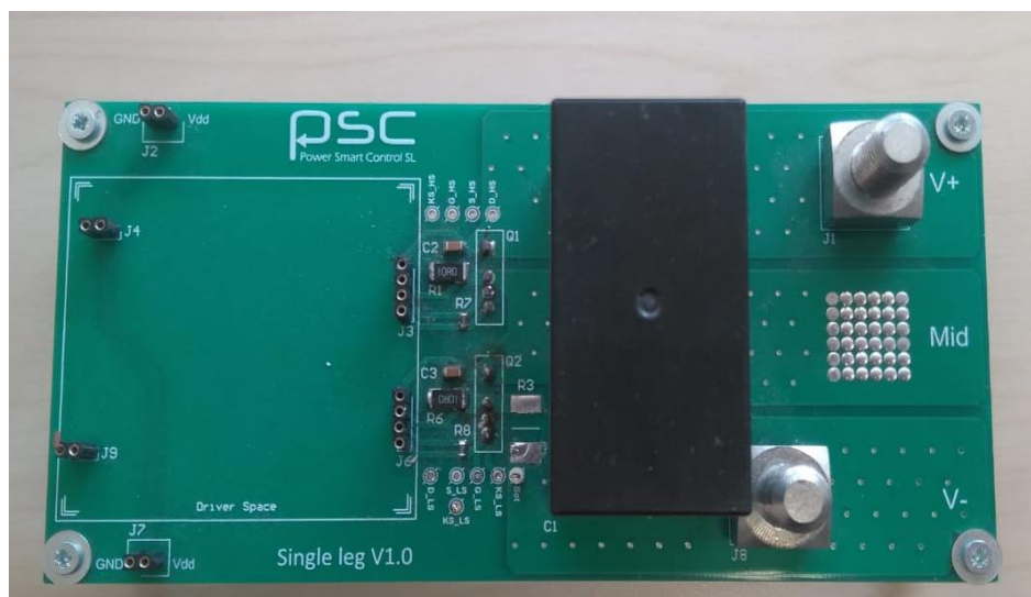
Figure 6: Double pulse test board
